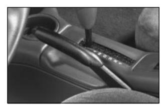
The parking brake lever is located between the bucket seats.
